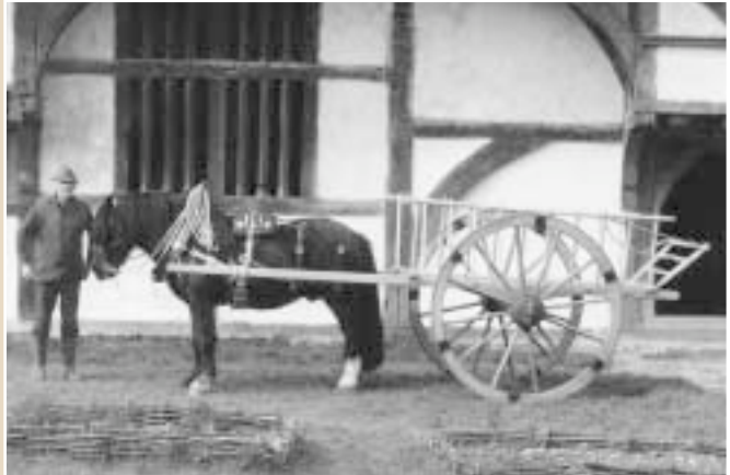
The replica medieval cart made for the Bayleaf Medieval Farmstead project by Emsworth wheelwright Keith Randall, scaling off measurements from the Luttrell Psalter. The 14 hands high Dales stallion, Babar, fitted perfectly between the shafts – practical proof of the size of horses prevalent at this period.
