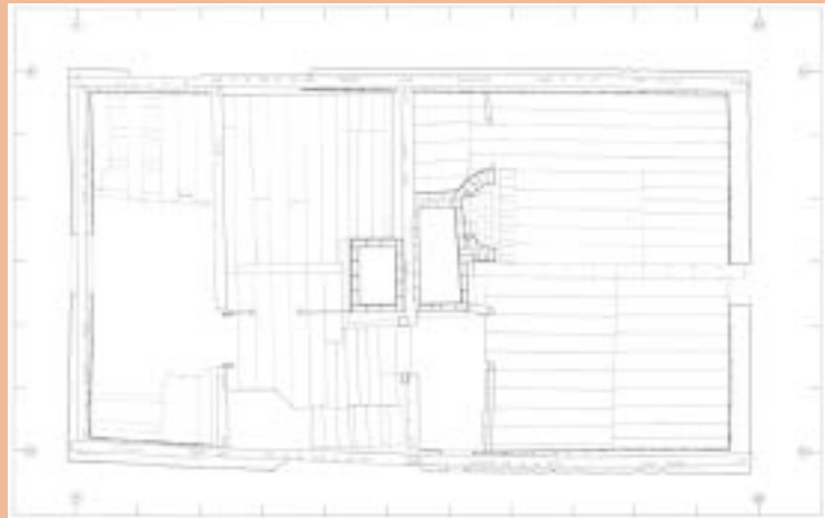
Below One of the record drawings from the dismantling, taken at the level of the upper floor and showing the soffit of the medieval timbers in reflected plan.
