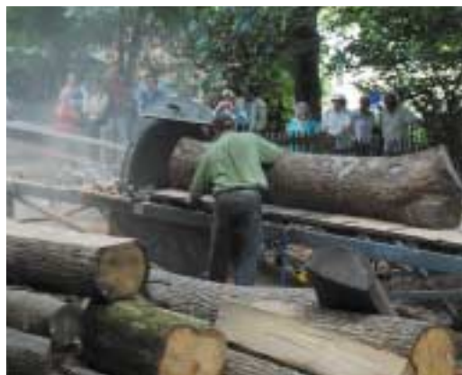
Steam sawing under way in the woodyard during the Steam Festival. Ash logs were swung onto the sawbench using the restored timber crane, where they were converted into planks for use in building restoration.
