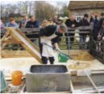
Gerard Lynch demonstrating lime-slaking outside Whittaker's Cottages. Dr Lynch also teaches the museum's courses on traditional and gauged brickwork.
