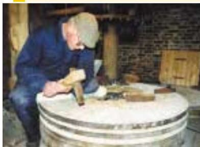
Robert Demaus dressing the mill's stones, a vital maintenance task to ensure the efficient production of flour, and below repairing the timber work at the mill leet.
